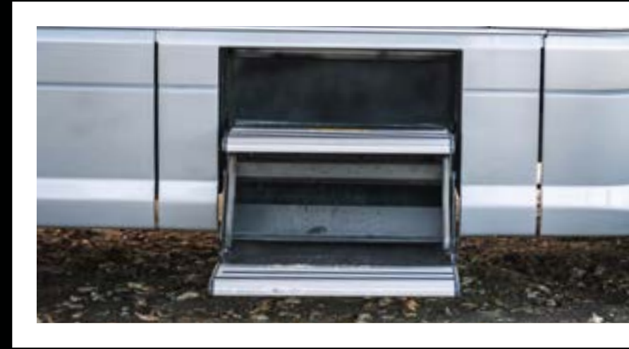
1 The powered step automatically extends and retracts when the door opens.
